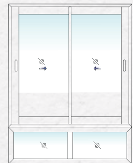
2T+2G SHUTTER SLIDING + BOTTOM FIXED WITH CENTER MULLION WINDOW
