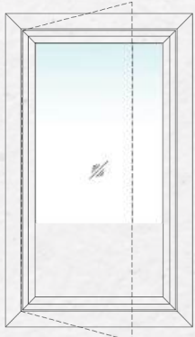
SINGLE SHUTTER OUTSIDE OPENING SIDE HUNG WINDOW
