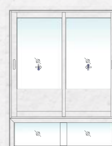
2T+2G shutter sliding + bottom Fixed with center mullion window
